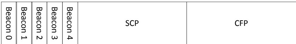
Figure 24 – Structure of a MAC Frame
